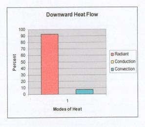
Radiant mode of heat transfer accounts for 93% of the downward flow of heat while the conduction mode of heat transfer accounts for 5%-7% and the convection mode of heat transfer is zero.
