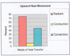
The radiant mode of heat transfer accounts for 50%-75% of the upward flow of heat while the conduction mode of heat transfer accounts for 5%-7% and the convection mode of heat transfer accounts for up to 45%.
