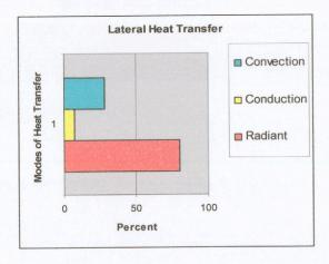
The radiant mode of heat transfer accounts for 65%-80% of the lateral (sideways) flow of heat while the conduction mode of heat transfer accounts for 5%-7% and the convection mode of heat transfer accounts for up to 15%-28%.
